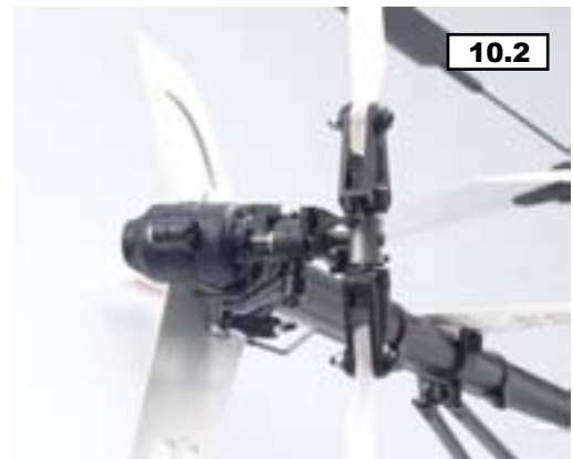
Guides should be helping the pushrod keep it's shape when being flexed. All 3 guides may not have to be used.
